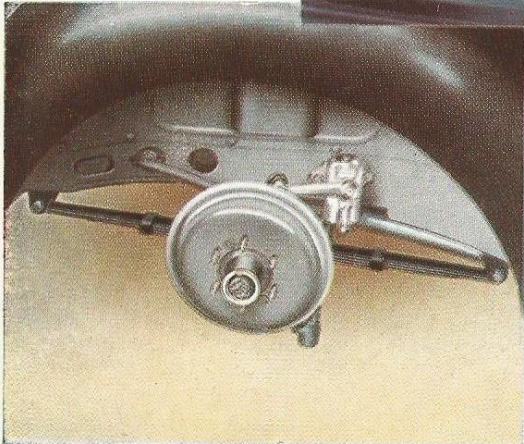
Reliable semi-elliptic springs of excellent length, controlled by up-to-date hydraulic shock absorbers, ensure the maximum comfort combined with safety.
